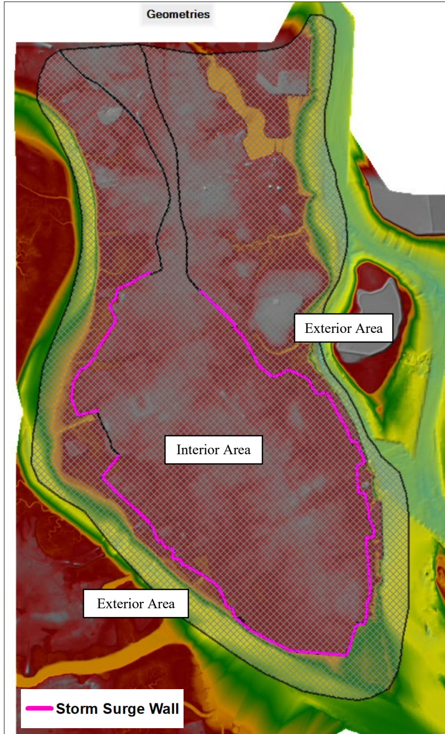
Figure 3.3.2 CSRM HEC-RAS Model with Storm Surge Wall Alignment
