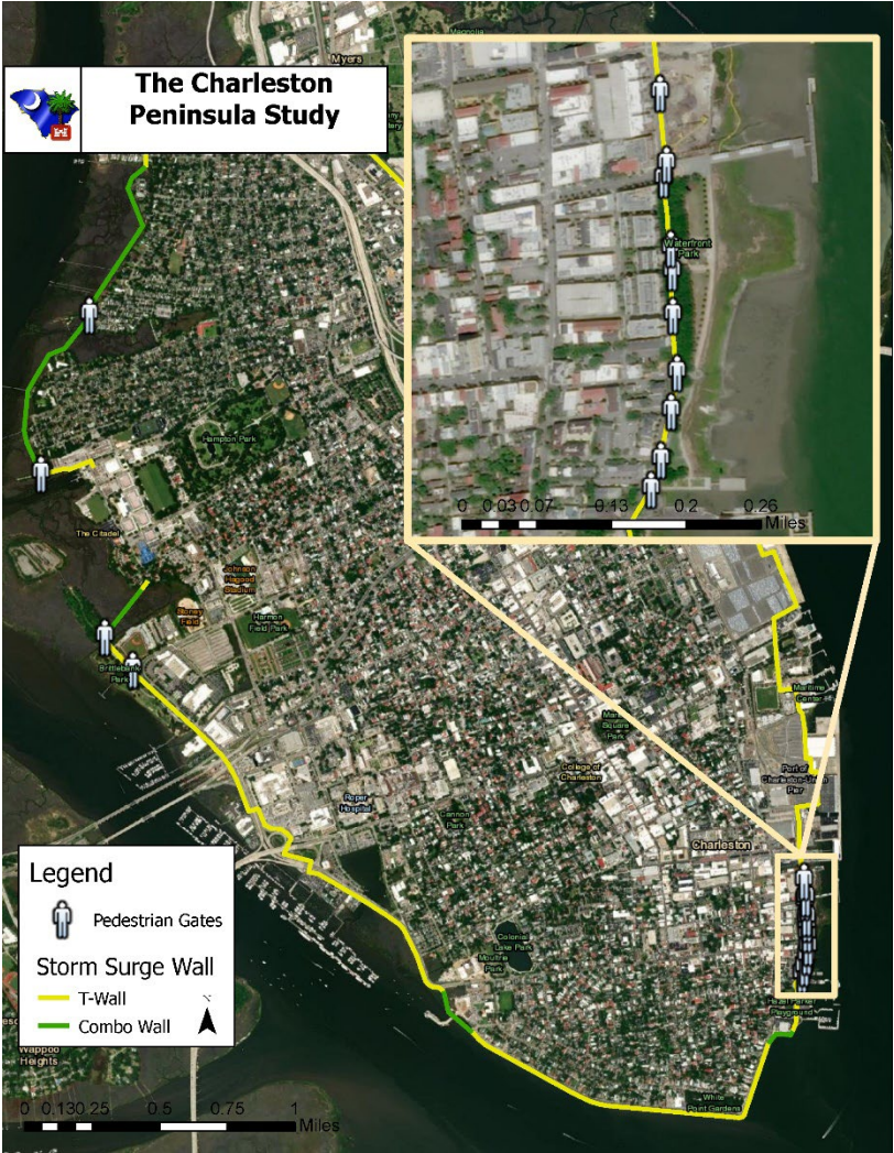
Figure 5.6.9 Pedestrian Gate Locations
