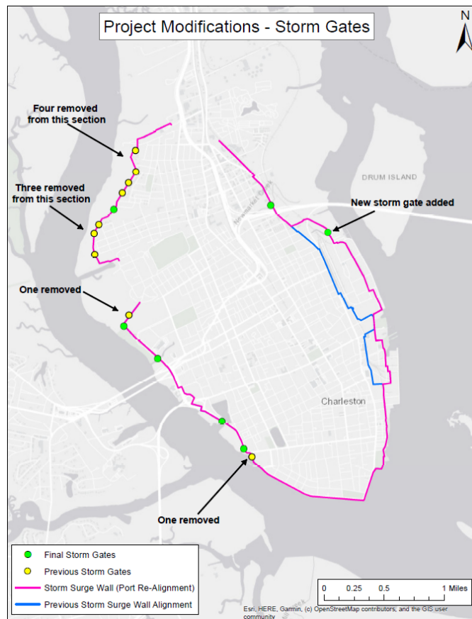
Figure 5.2.1 TSP Project Modification – Storm Gates
