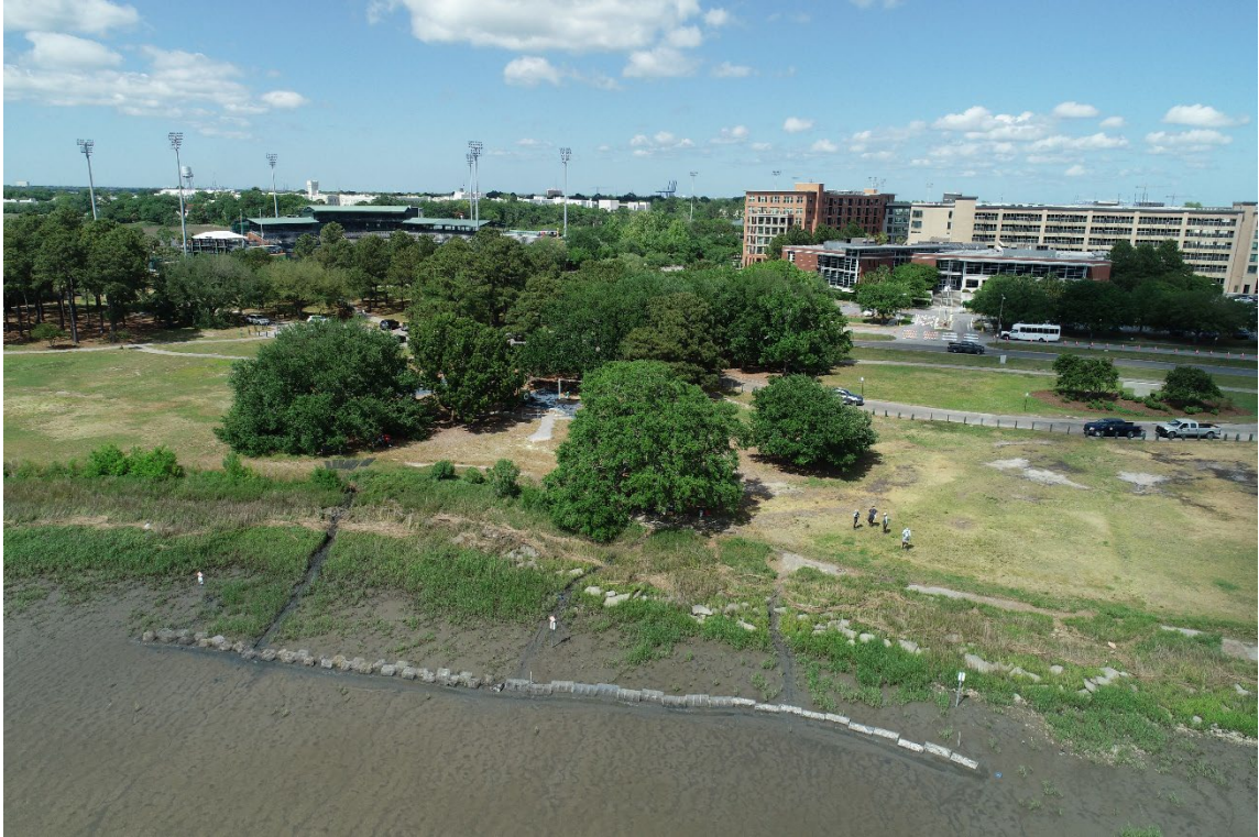
Figure 6.4. Living shoreline sills constructed with different manufactured wire reef configurations along the Ashley River by Brittlebank Park. There are also some segments of bagged oyster shell reef sills in the vicinity (not shown in photo). Source: photo courtesy of SCDNR.
