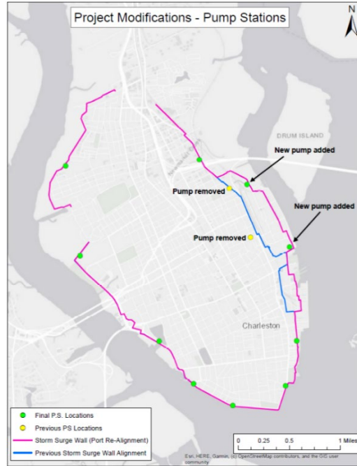
Figure 5.2.2 TSP Project Modification – Pump Stations
