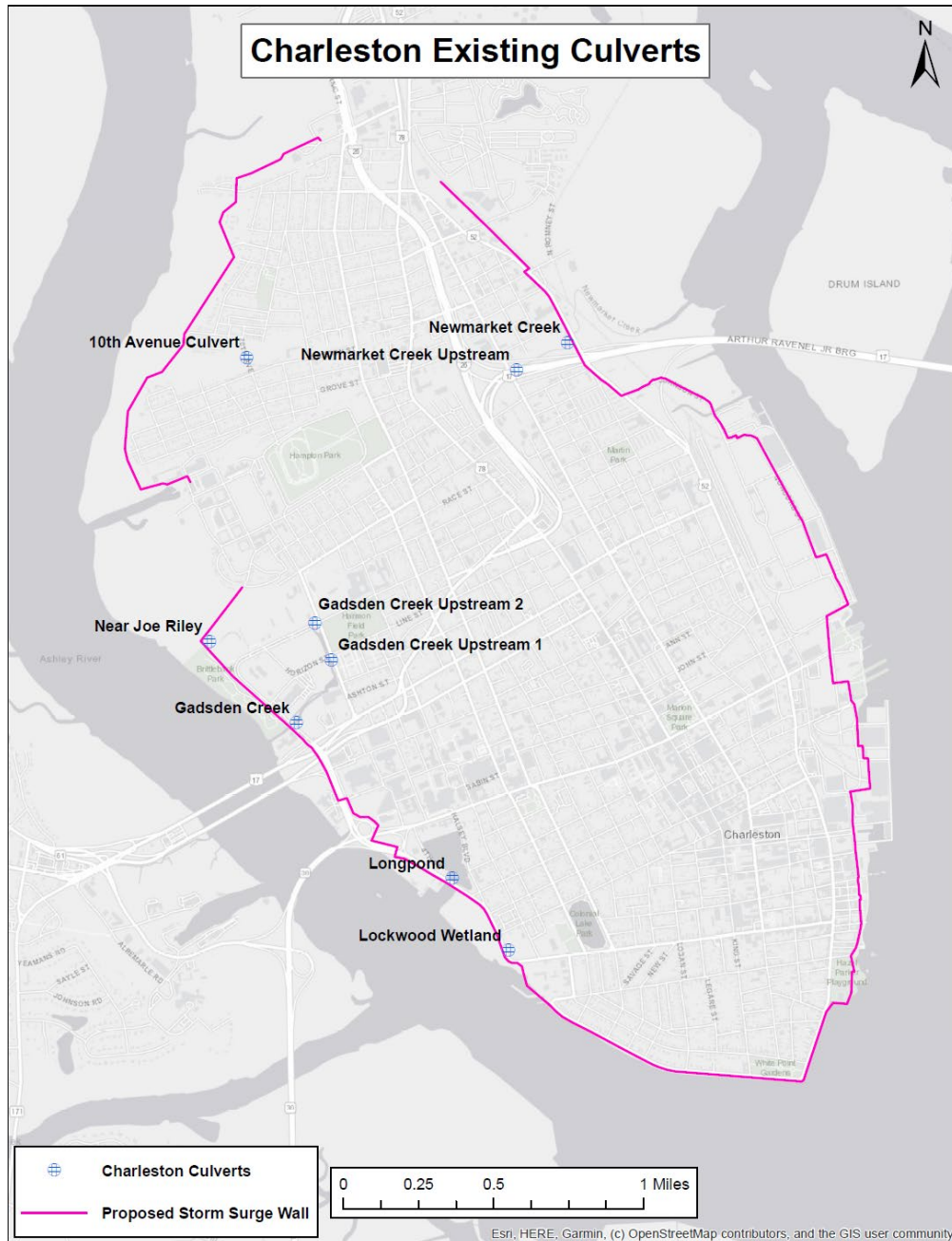
Figure 5.10.4 Charleston Existing Culverts
