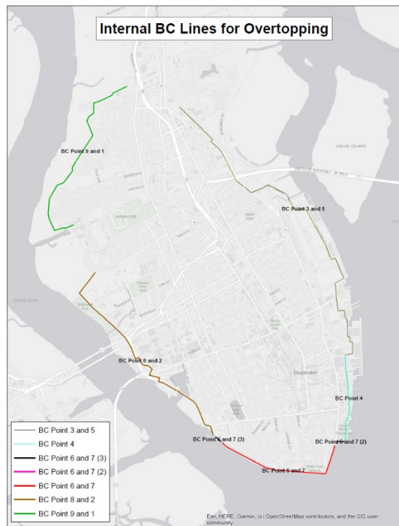
Figure 10. Internal BC Lines for Wave Overwash
