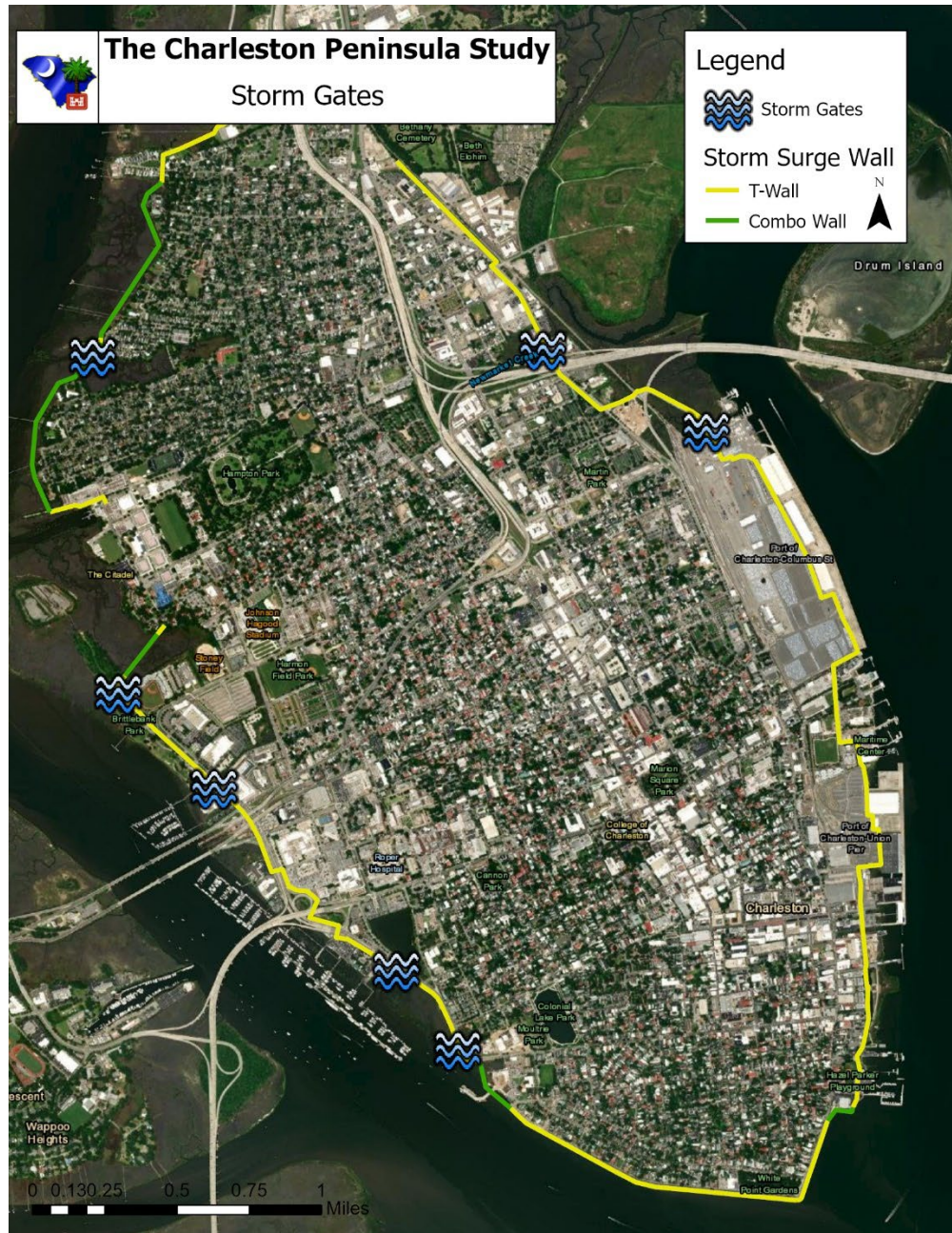
Figure 5.6.10 Locations of Storm Gates
